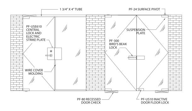
**SECTION - RECESSED** DOOR CHECK AT THE TOP WITH SUSPENSION PLATE AT TOP AND BOTTOM
